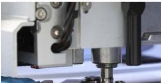
f. Open the grey lever and remove the O-Ring (by using the tweezers) from pipetting channel. Note: If required, repeat cutting process until O-Ring is cut completely and can be removed.
