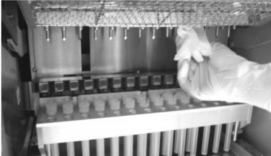
5. Close the EZ1 door and press **ENT**. The piercing unit returns to its original position and the manual operation screen appears.
