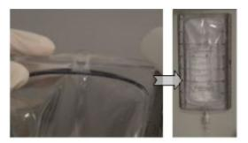
Connect vacuum side of tubing to SEC by slipping the quick-connect fitting into the vacuum port on SEC labeled "to M-VAC"
