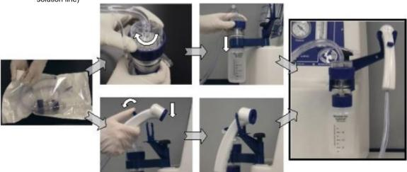
4. Open extension tubing by tearing at the notches on the side of the pouch. Attach solution line fitting to the M-Vac fitting on the M-Vac. Lightly attach vacuum tubing
